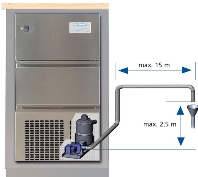
Fig. 5.4: Ice cube maker modell W55 LE/ W with optional condensation water pump
